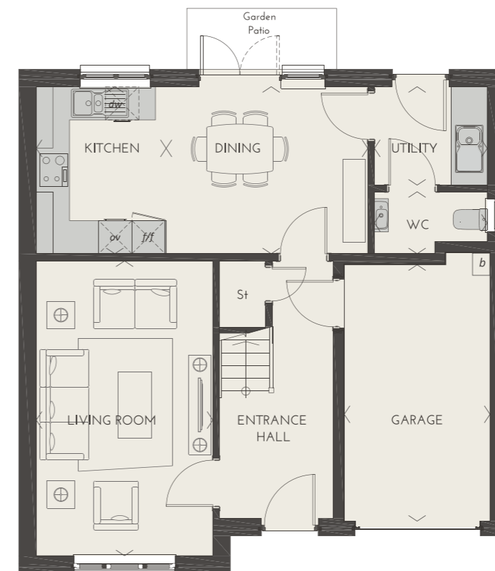
Legend: b - boiler ff - tall integrated fridge freezer ov - tall integrated oven and optional microwave dw - optional integrated dishwasher St - store
