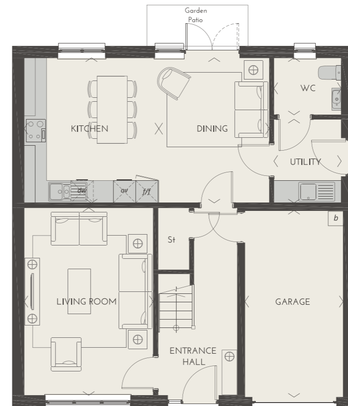
Legend: b - boiler fff - tall integrated fridge freezer ov - tall integrated oven and optional microwave dw - optional integrated dishwasher St - store
