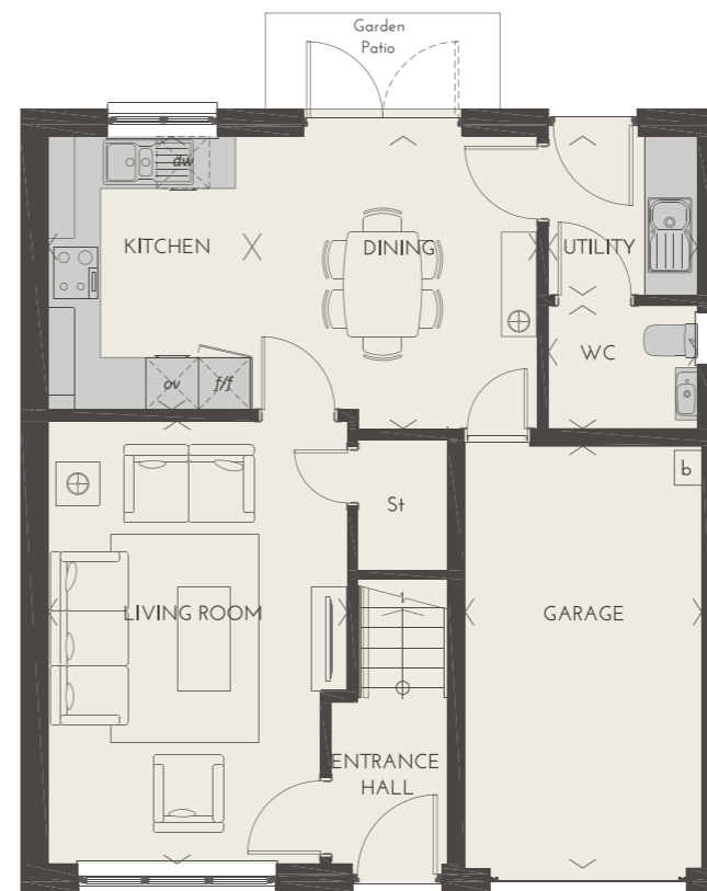
Legend: b - boiler f/f - tall integrated fridge freezer ov - tall integrated oven and optional microwave dw - optional integrated dishwasher St - store
